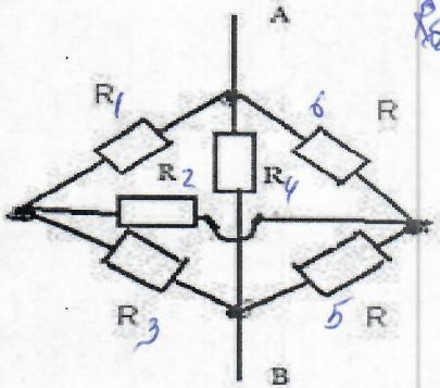
$$\frac{1}{R_{AB}} = \frac{1}{R_1} + \frac{1}{R_2} + \frac{1}{R_3} + \frac{1}{R_4} + \frac{1}{R_5}$$
